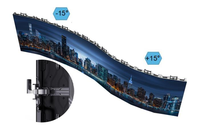
1 Press the tab . 2 Lock the curve lock.
