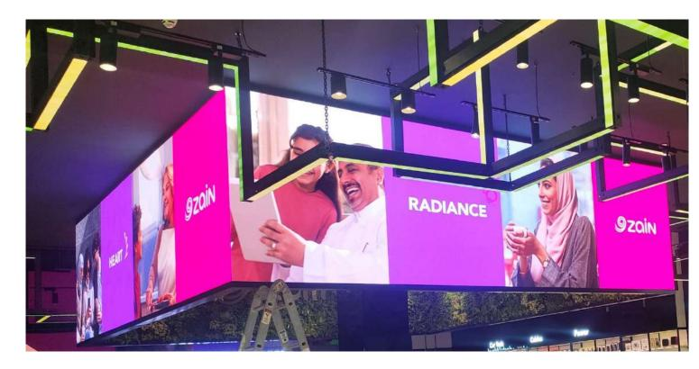
Moreover, this product's adaptable design allows for the creation of cube shapes, expanding its versatility even further. By preserving the 45-degree cutting angle within the product structure, users can seamlessly construct cube configurations without the hassle of cabinet alterations, streamlining the process and offering greater convenience in achieving unique display arrangements.
