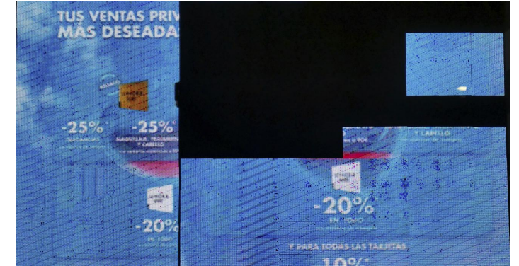
Module connector, power cable or Hub card issue
